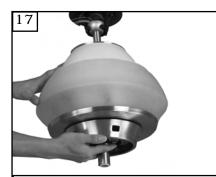
Raise fan with downrod assembled to the ceiling bracket and hang fan assembly. Be sure to rotate the downrod ball so that the notch in the bracket engages the slot in the ball.
